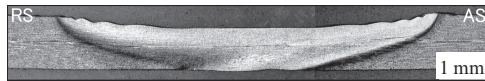
RS: Retreating side AS: Advancing side (a) Condition; Tool rotation speed: 200 \text{ min}^{-1} - Travel speed: 200 \text{ mm} \cdot \text{min}^{-1}
